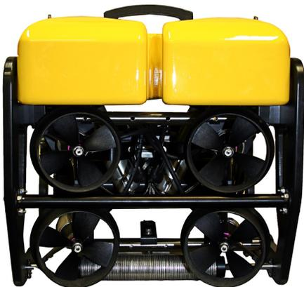
The **Chinook** is an industrial grade inspection ROV with a wide range of capabilities. Explore depths up to 300 m (1,000 ft) with the standard vehicle or 600 m (2,000 ft) with the deep water version.
